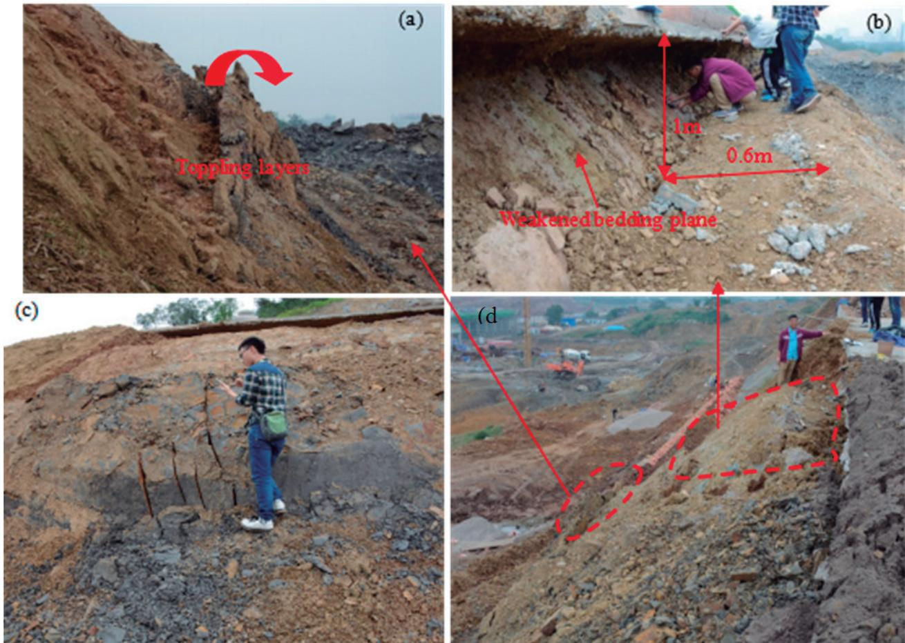
**Figure 5.** The complex slope failure taking place in situ. (a) toppling of the rock mass in the lower part; (b) sliding along the bedding plane in the upper part; (c) cracking of the slope face due to the push of sliding rock columns in the upper part. (d) Panoramic view of the landslide.
