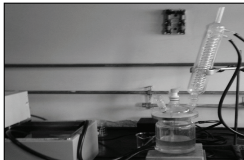
Figure 1. Jacketed reactor with reflux condenser. The thermostat is on the left hand side
