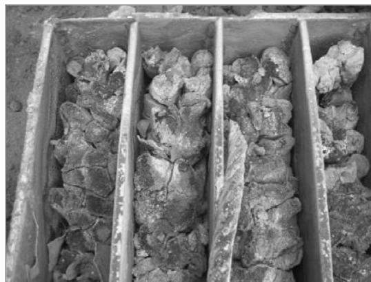
Figure 5. Coked briquettes in a box having divisions in a hearth furnace
