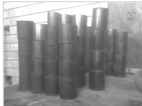
**Figure 3. Briquettes obtained from ultrafine coal particles****Table 2. Briquette compressive and impact strength tests**
