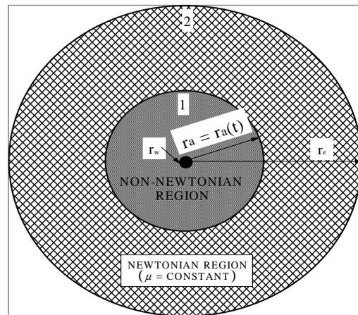
Figure 1. Composite non-Newtonian/Newtonian radial reservoir
