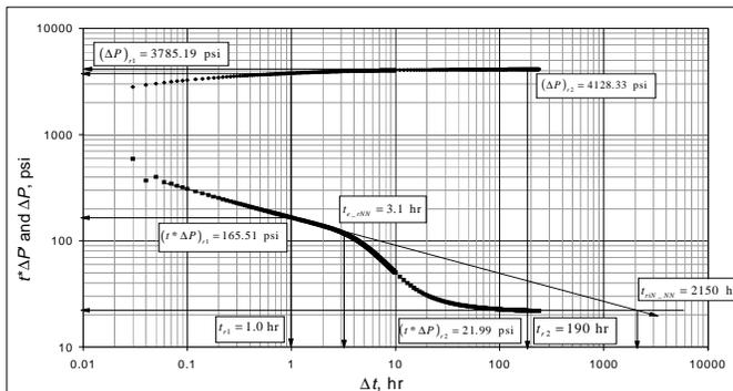
Figure 3. Pressure and pressure derivative for example 1
