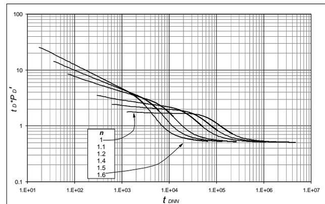
Figure 2. Newtonian dimensionless pressure derivative pattern for *r<sub>o</sub>* = 120 ft
