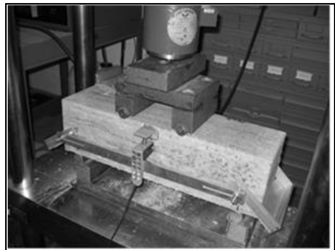
Figure 5. Test set-up for the three-point bending test
