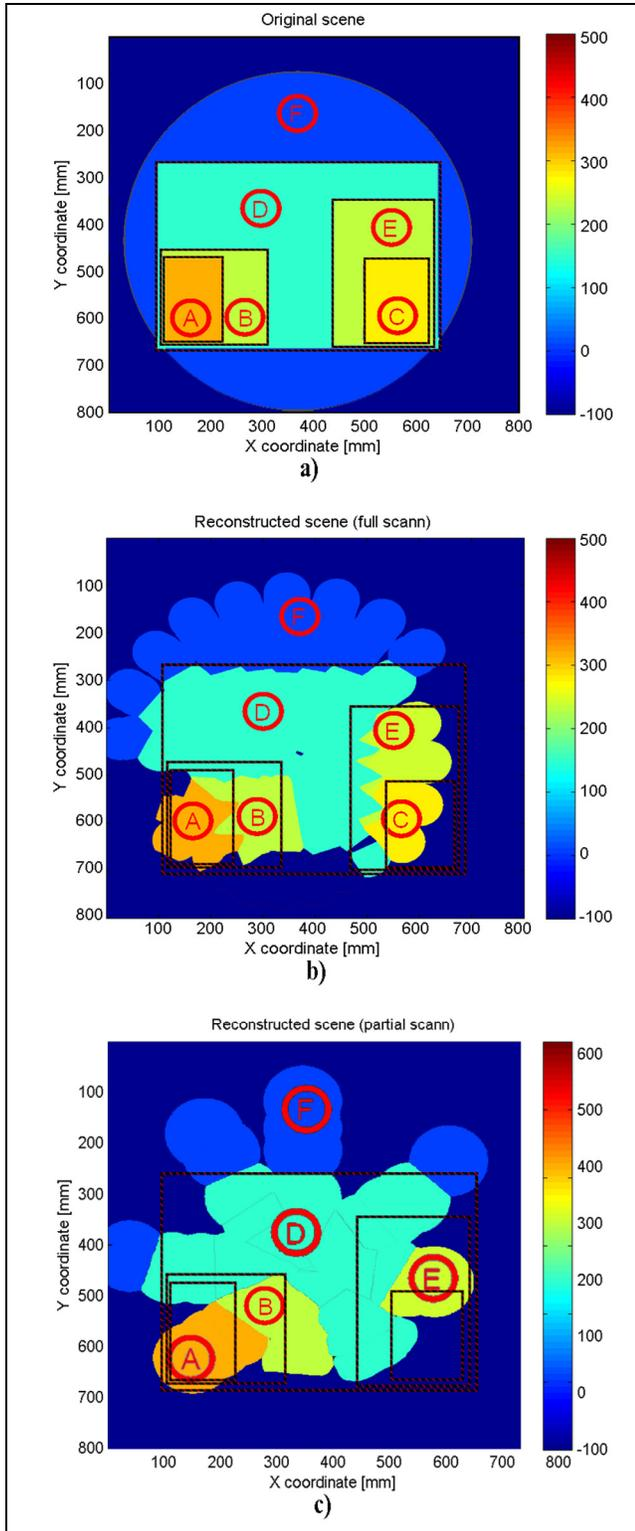
Figure 4. Depth reconstruction, ideal (top), full scan (middle), partial scan (bottom)
