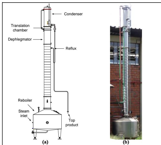
Figure 1. Batch still (a) layout and (b) prototype.
