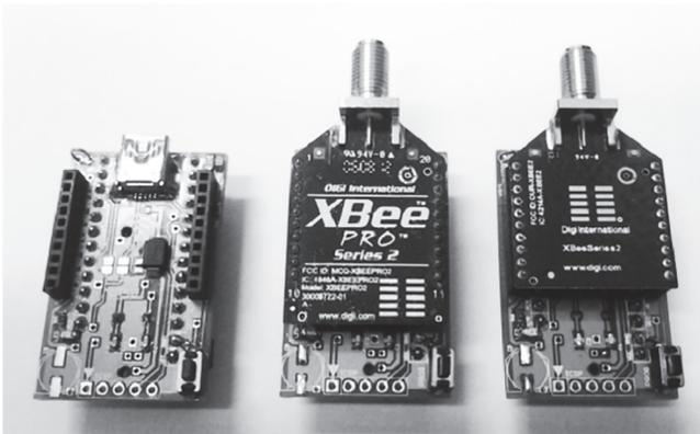
Figure 2. Data acquisition boards, FFD and RFD transceivers.
