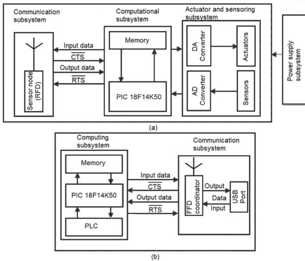
Figure 1. EEWES: (a) RFD block diagram. (b) FFD block diagram.
