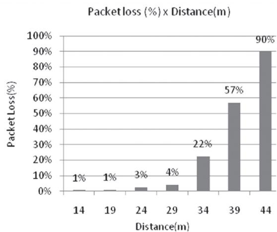
Figure 7. Packet loss (%) x Distance(m) in 10 rounds.
