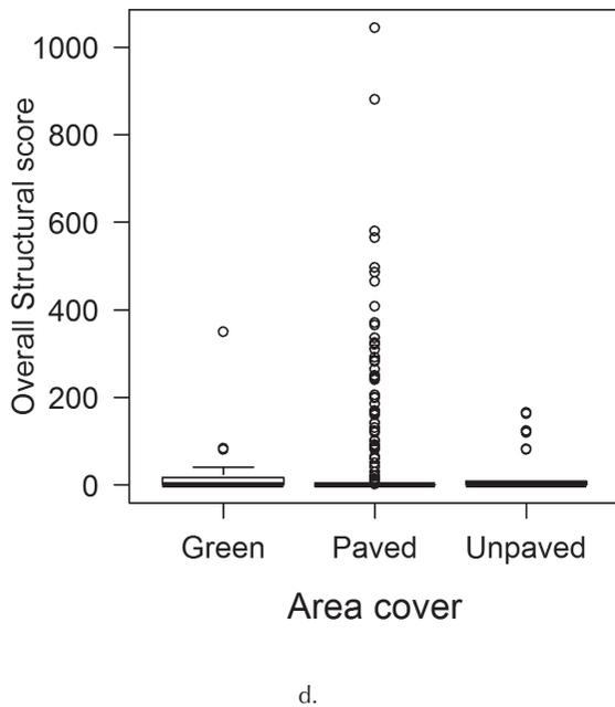
**Figure 4.** Models in Group I. Structural score of pipe = f(x<sub>i</sub>); a) x<sub>1</sub>: material, b) x<sub>2</sub>: diameter, c) x<sub>3</sub>: xarea type y and d) x<sub>4</sub>: network type. **Source:** Authors
