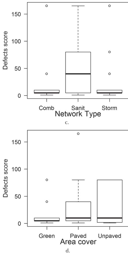
**Figure 7.** Other models in Group III. Significant associations with other types of failures: 1112: Crack or fracture, 1123: Deposits stuck, sediment or soil entering, 1113: Breakage or collapse, 1121: Obstruction by connection.
