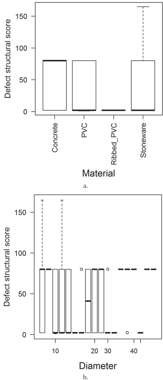
**Figure 5.** Models in Group II. Individual defect score =  $f(x_i)$ ; a) x1: material, b) x2: diameter, c) x3: network type and d) x4: area type.
