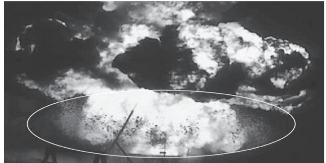
**Figure 17.** Explosion of slab 2. The circle highlights the EPS being burned. Image recorded 9,6 m after trigger.
