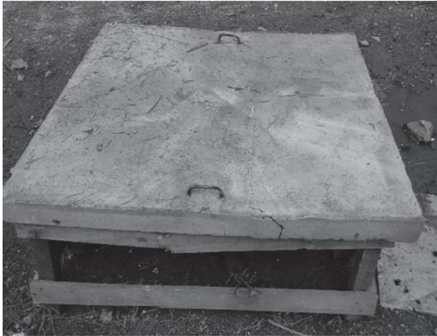
**Figure 15.** Slab 3 after test.
