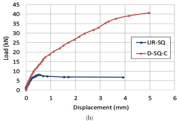
**Figure 6.** Load vs. Lateral Displacement: (a) Slender walls; (b) Squat walls.
