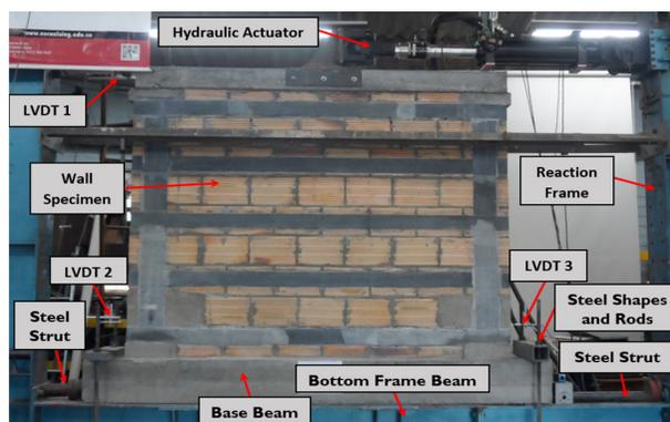
Figure 5. Overall view of the test setup.
