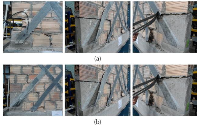
**Figure 8.** Failure mode of the diagonally reinforced walls: (a) Slender walls; (b) Squat walls.
