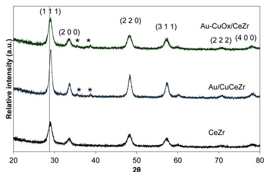
**Figure 4.** XRD patterns of CeZr support and the catalysts Au-CuO<sub>x</sub>/CeZr and Au/CuCeZr \*CuO.
