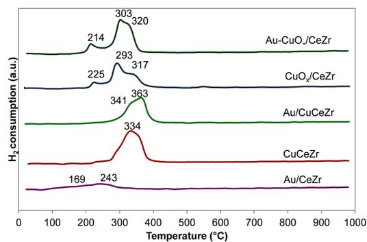
**Figure 1.** TPR- $\text{H}_2$  patterns of the bimetallic catalysts Au- $\text{CuO}_x/\text{CeZr}$ , Au/CuCeZr; the monometallic catalysts  $\text{CuO}_x/\text{CeZr}$ , CuCeZr, Au/CeZr; and the CeZr support.
