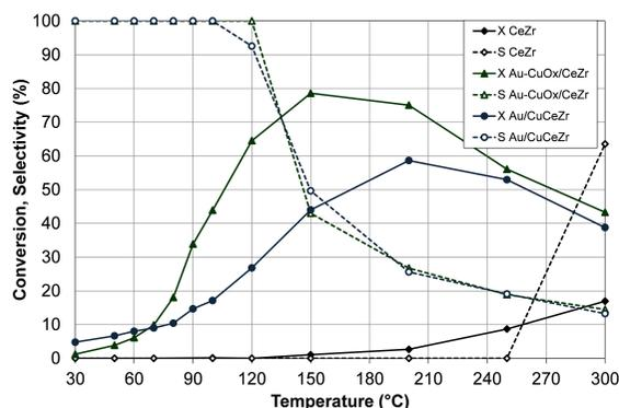
**Figure 5.** CO conversion (X, filled symbols) and selectivity to CO<sub>2</sub> (S, empty symbols) of CeZr, Au-CuO<sub>x</sub>/CeZr and Au/CuCeZr. Feed stream: 2 % CO, 2 % O<sub>2</sub>, 50 % H<sub>2</sub> and He (balance).
