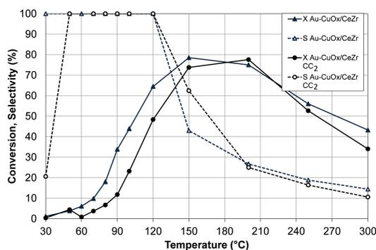
**Figure 7.** Effect of CO<sub>2</sub> on the CO conversion (X, filled symbols) and selectivity to CO<sub>2</sub> (S, empty symbols) of Au-CuO<sub>x</sub>/CeZr. Feed stream: 2 % CO, 2 % O<sub>2</sub>, 2 % CO<sub>2</sub>, 50 % H<sub>2</sub> and He (balance).
