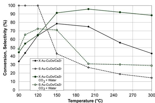
**Figure 8.** Effect of water and CO<sub>2</sub> on the CO conversion (X, filled symbols) and selectivity to CO<sub>2</sub> (S, empty symbols) of Au-CuO<sub>x</sub>/CeZr. Feed stream: 2 % CO, 2 % O<sub>2</sub>, 2 % CO<sub>2</sub>, 3 % H<sub>2</sub>O, 50 % H<sub>2</sub> and He (balance).
