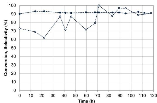
**Figure 9.** Catalytic stability of the Au-CuO<sub>x</sub>/CeZr. Evaluation of the CO conversion (X, filled symbols) and selectivity to CO<sub>2</sub> (S, empty symbols) with addition of CO<sub>2</sub> and water. Feed stream: 2 % CO, 2 % O<sub>2</sub>, 2 % CO<sub>2</sub>, 3 % H<sub>2</sub>O, 50 % H<sub>2</sub> and He (balance).
