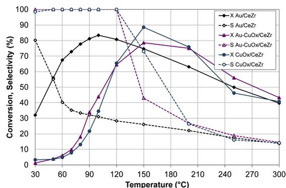
**Figure 6.** CO conversion (X, filled symbols) and selectivity to CO<sub>2</sub> (S, empty symbols) of Au-CuO<sub>x</sub>/CeZr with respect to Au/CeZr and CuO<sub>x</sub>/CeZr. Feed stream: 2 % CO, 2 % O<sub>2</sub>, 50 % H<sub>2</sub> and He (balance).
