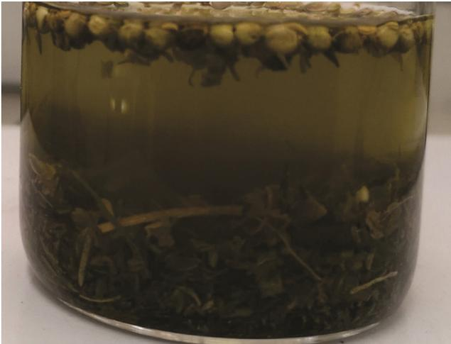
**Figure 5.** Lixiviate obtained by extraction with ethanol in a single stage at 20 °C
