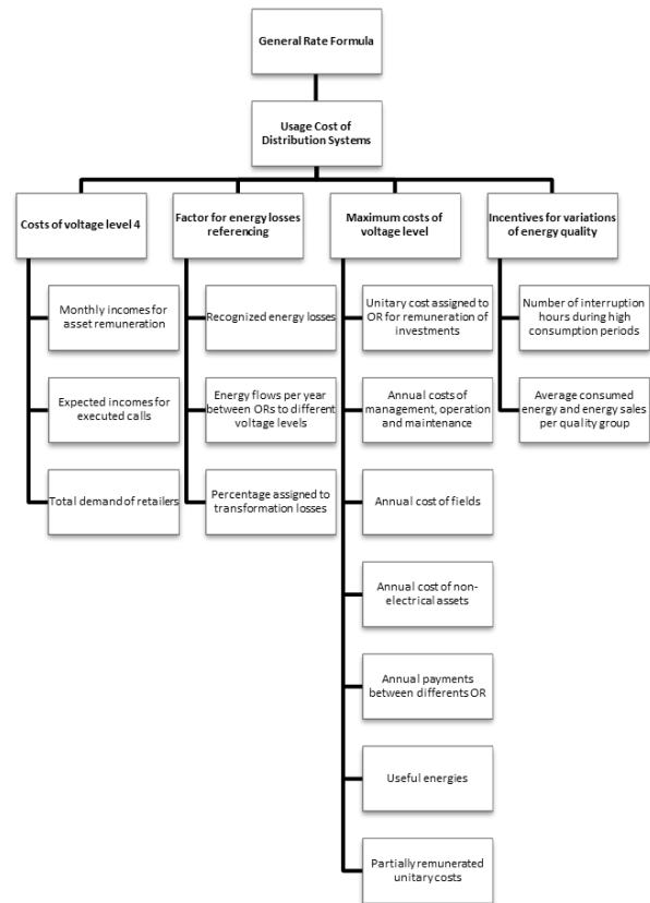
Figure 1. Parameters that affect the calculation of Usage Costs of Distribution Systems for voltage levels 2, 3 and 4.
