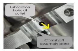
Figure 6. Oil lubrication hole and camshaft bore.
