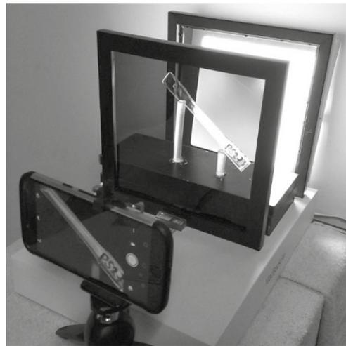
Figure 2. Experimental setup for photoelasticity tests.
