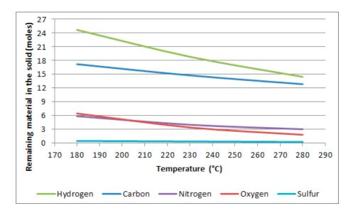
**Figure 5.** Variation of the remaining material in the tanned wastes after thermal treatment in the 180°C – 280°C range.
