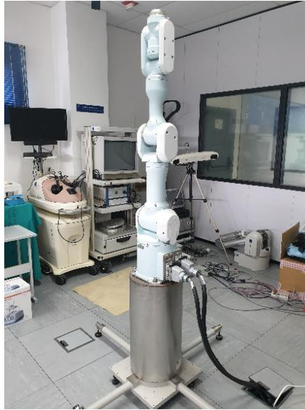
FIGURA 2. BRAZO INDUSTRIAL PA10 UTILIZADO.
