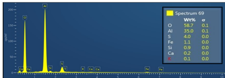
Figure 15. Elemental chemical analysis of pitting in the OPGWs
