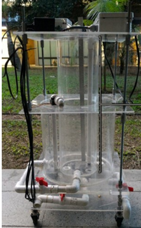
Figure 1. Level plant with interconnected concentric tanks
