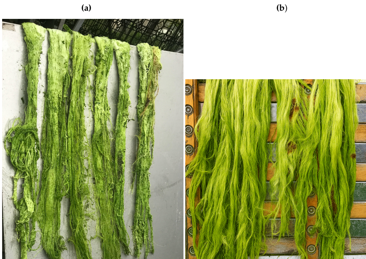
Figure 11. Fiber obtained after decortication in the proposed machine a) as produced by the machine and b) after washing and brushing
