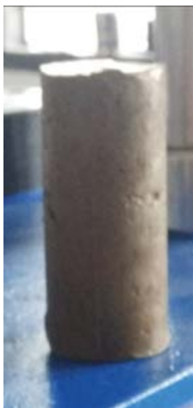
Fig. 1. SOIL SAMPLE PREPARED FOR UCS TESTING
