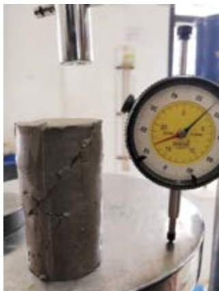
Fig. 2. SOIL SAMPLE DURING UCS TESTING
