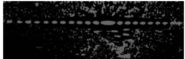
Figure 10. Thresholding the image captured of diffraction pattern RS1.
