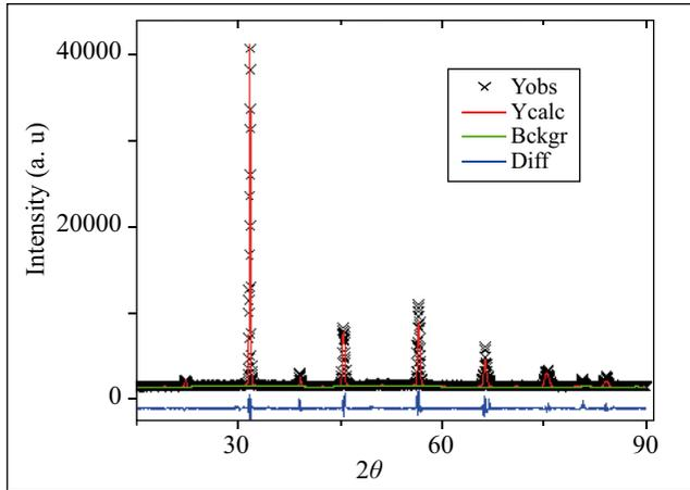
**Figure 2.** X-ray diffraction pattern for  $\text{Sr}_2\text{SbMnO}_6$  ceramics after Rietveld refinement of the crystal structure at room temperature.
