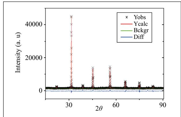
**Figure 4.** Observed, calculated and difference plots of the X-ray diffraction pattern for  $\text{Sr}_2\text{SbMnO}_6$  after Rietveld refinement at 600 °C.
