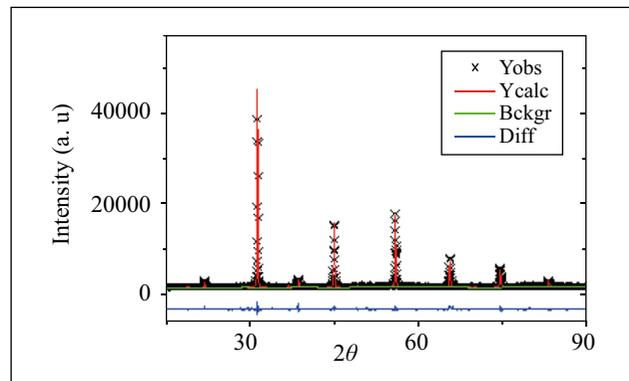
**Figure 5.** Rietveld refinement of the X ray diffraction pattern for  $\text{Sr}_2\text{SbMnO}_6$  ceramics at 800 °C.
