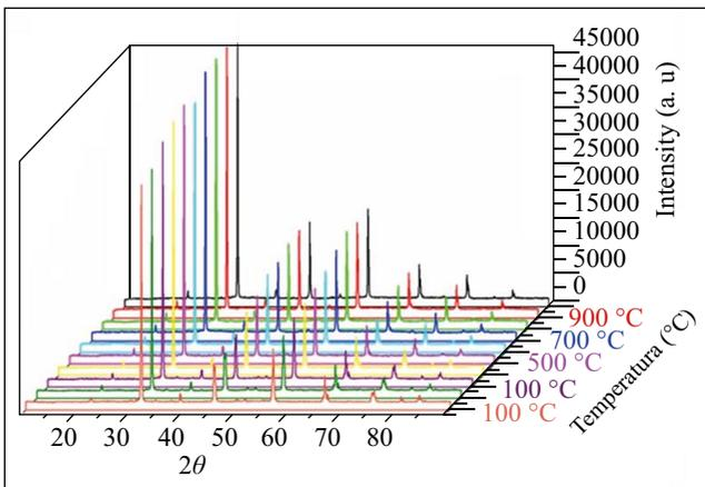
**Figure 3.** Temperature evolution of the X ray diffraction pattern of  $\text{Sr}_2\text{SbMnO}_6$ .
