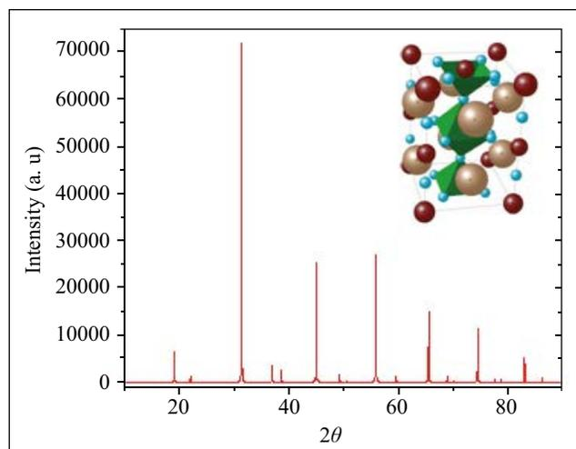
**Figure 1.** Crystal structure of the tetragonal P4/mnc structure of perovskite material Sr<sub>2</sub>SbMnO<sub>6</sub>.
