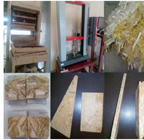
Figure 12. Manufacturing process of test samples and board
