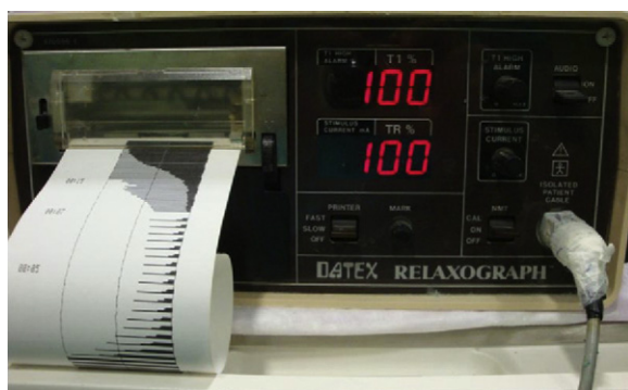
Fig. 2 – Electromyograph. Relaxograph NMT Monitor (Datex Instrumentarium Corp., Helsinki, Finland). Recording strip with real time TOF.
