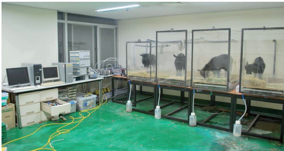
Figure 2. A photo of the respiration-metabolism chamber system for small ruminant animals.
