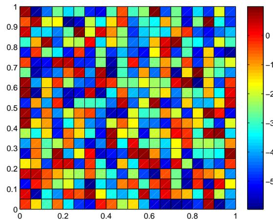
**Figure 2.** Random isotropic permeability distribution in logarithmic scale.
