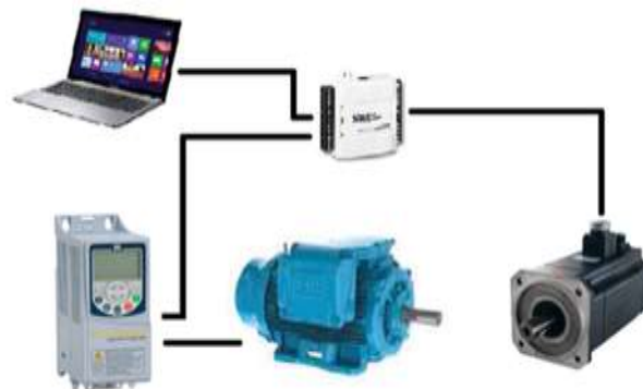
Fig. 2. Arrangement of wind turbine emulator equipment.
