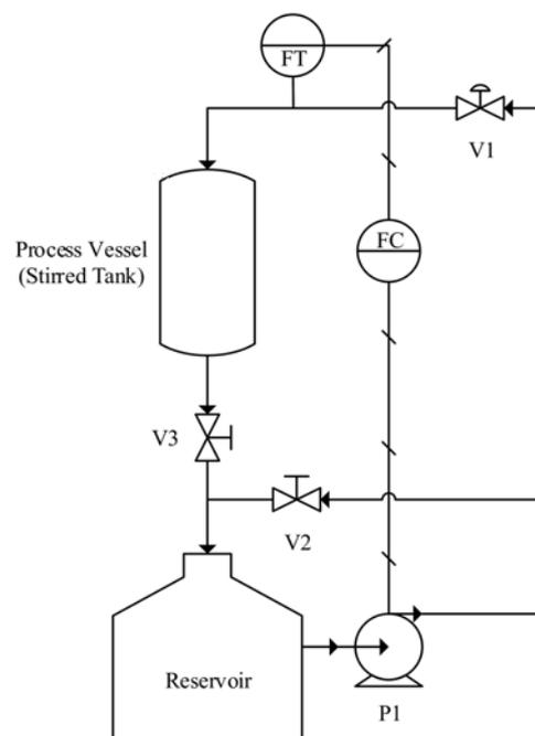
**Figure 3** P&ID of the pump-based control strategy
