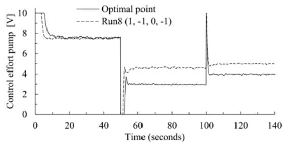
**Figure 13** Pump control effort for CCF-Run8 (1, -1, 0, -1) and Optimal point
