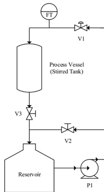
**Figure 2** Piping and instrumentation diagram of the process
