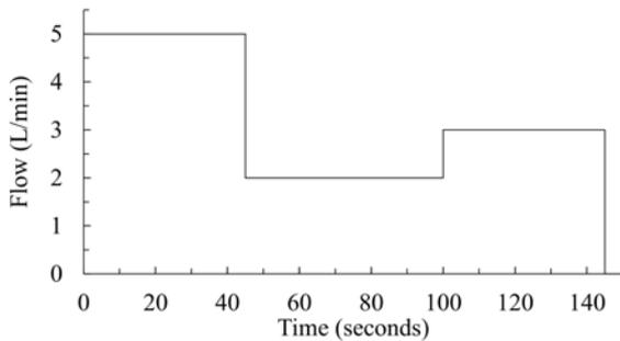
Figure 5 Setpoint sequence for flow control loops
