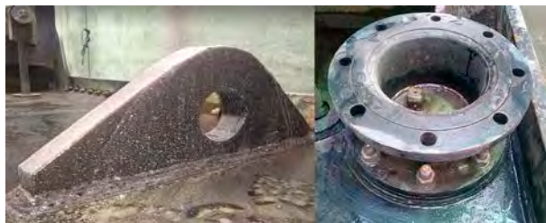
Figure 5 Lifting handles (a), and Accelerometers chamber (b)
