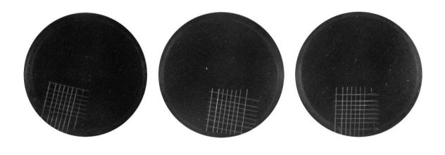
Figure 4 Picture of the CPF coatings after adhesion test. Samples were immersed for 1 month in 10<sup>-2</sup> M NaCl solution
