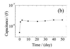
Figure 2 Evolution of the impedance parameters of the CPF coatings during immersion in 10<sup>-2</sup>M NaCl solution
