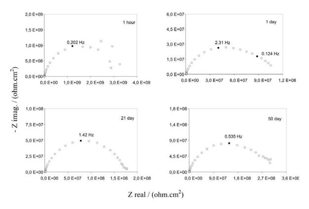
Figure 1 Impedance of CPF coating for different immersion times in 10<sup>-2</sup> M NaCl solution
