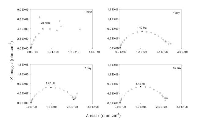
Figure 3 Impedance of the free-standing film of the CPF coatings at different immersion times in 10<sup>-2</sup> M NaCl solution
