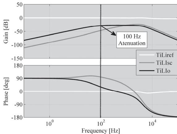
**Figure 5** Closed-loop frequency response of the inductor-current controlled system
