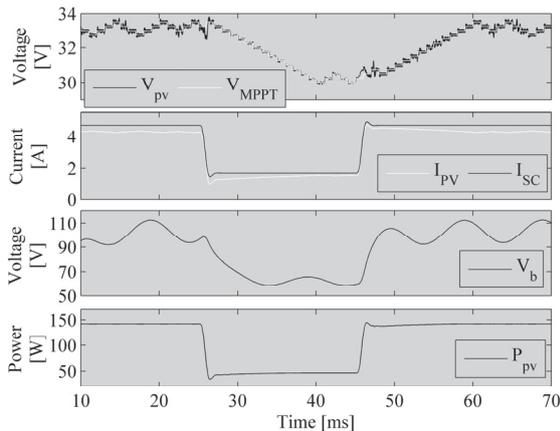
**Figure 12** Simulation of the single-controller voltage-regulated PV system
