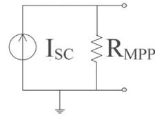
**Figure 3** PV panel small-signal model: Norton equivalent
