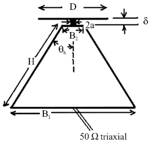
**Figure 2** Discone antenna.  $H$  = height of the cone,  $B_1$  = diameter of the cone,  $D$  = diameter of the disc,  $\theta_h$  = angle of opening of half a cone,  $B_2$  = wide of the apex of the cone,  $\delta$  = height of the insulating material between the disc and the cone and  $2a$  = wide of the insulating material
