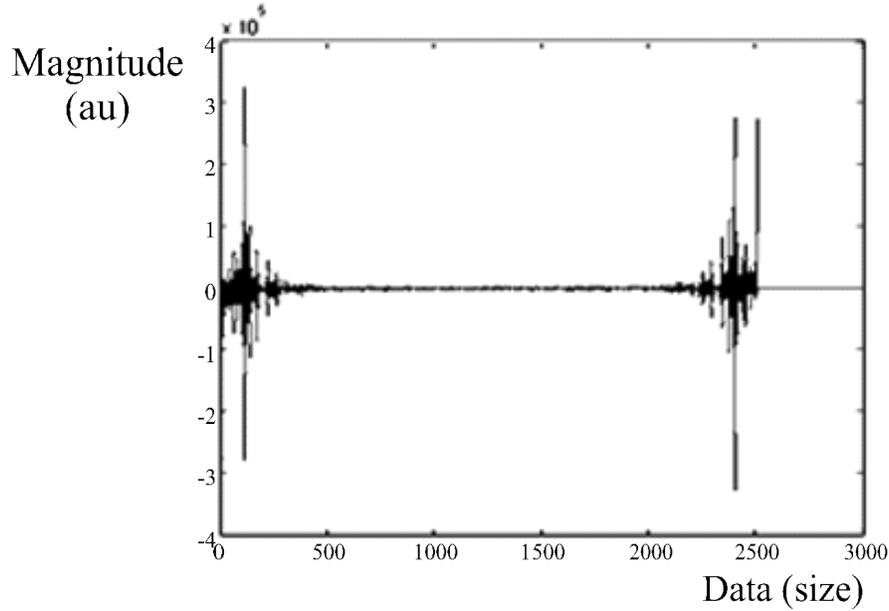
**Figure14** Difference between the Fourier coefficients of the signal of the transformer with respect to the pure signal of the insulator
