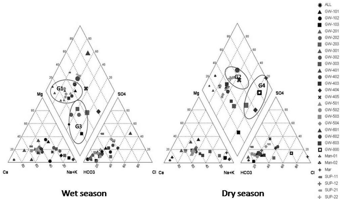
**Figure 5** Grouping of samples using Piper diagrams
