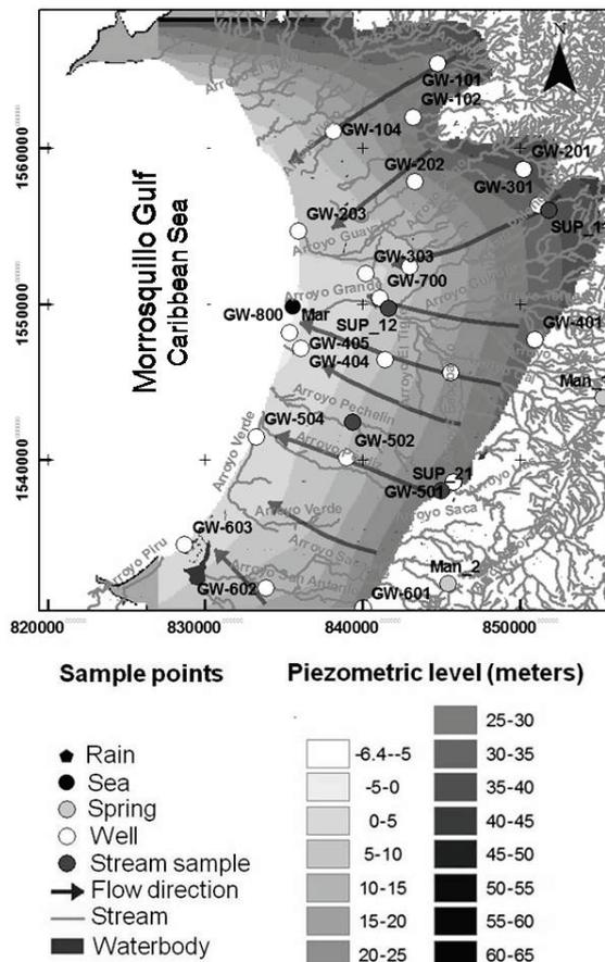
**Figure 3** Monitoring network, water table and flow lines
