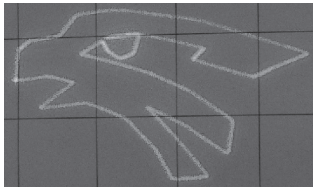
Figure 2 Experimental implementation for the decomposed Piecewise-Linear proposal. (a) LabView Front Panel screen in the LP20 galvo system. (b) Laser projection for the falcon- icon, \alpha =38 , \delta =0.1
