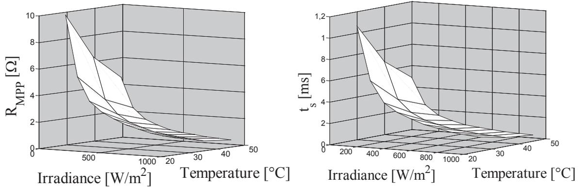
**Figure 10** Changes in the irradiance and the temperature, directly affects the settling time
