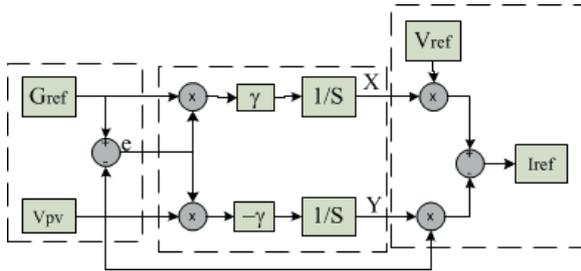
Figure 13 Block diagram of the adaptive controller
