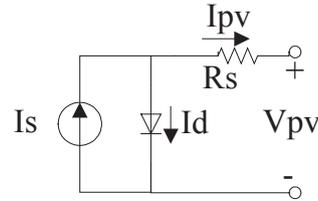
**Figure 2** Equivalent electrical circuit of a PV cell
