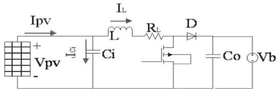
**Figure 1** PV system based on a boost converter
