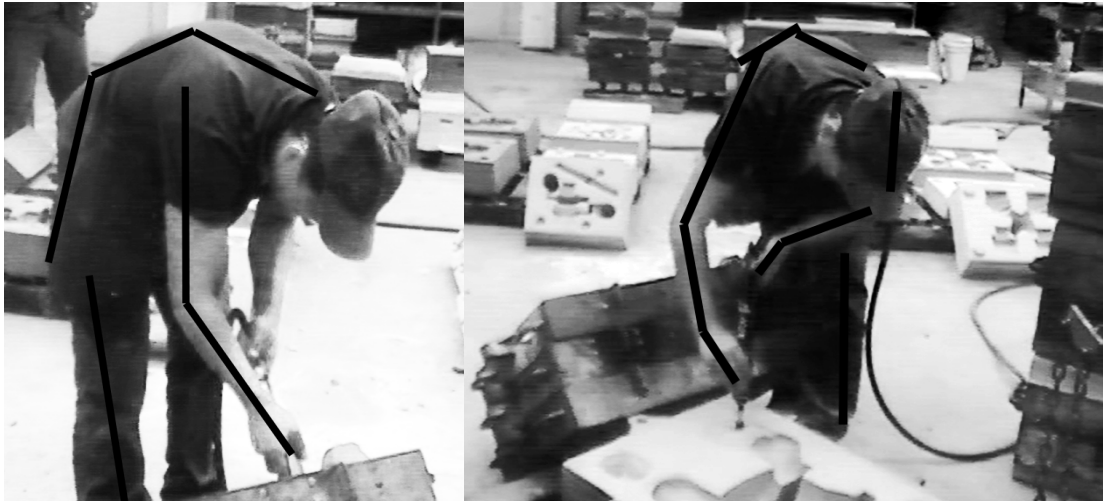
Figure 3 Example of postures analyzed by REBA in the finishing operation of molding
