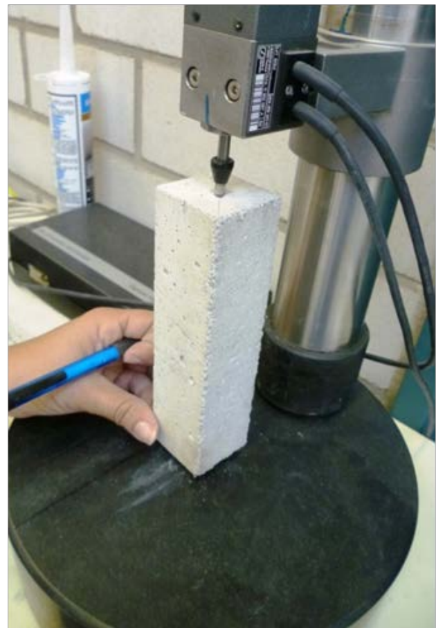
Figure 2 Device for the measurement of expansion in mortar prisms
