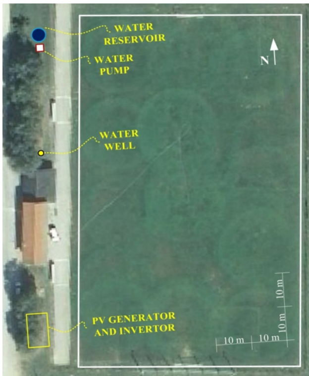
Figure 3 Irrigation system layout scheme (modified from [16])
