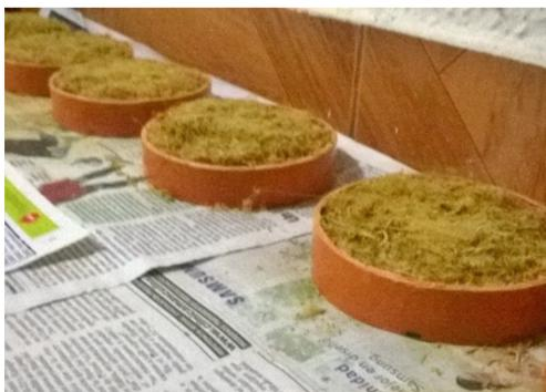
**Figure 2** Guadua test specimens
