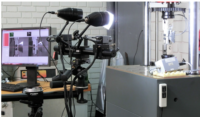
Figure 2 Experimental set-up for fatigue testing
