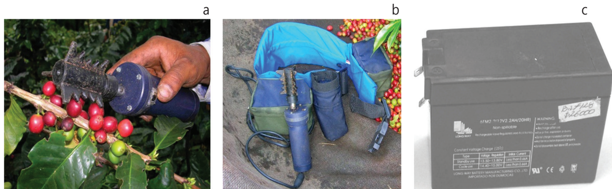
Figure 1. Equipment Alfa. a. actuator, b. harness and c. battery.
