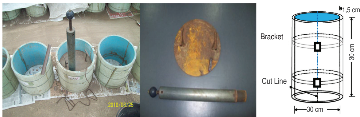
Figure 2. Containers of PVC and Proctor hammer.
