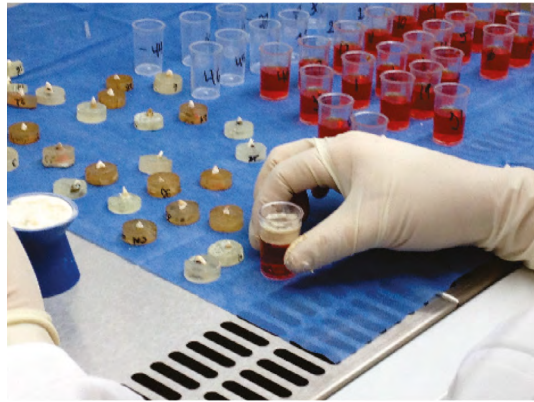
Figure 1. Assembly of tube (upper and lower chamber) and marker of bacterial presence (phenol red) in lower chamber
