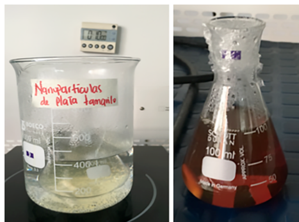
Figure 1. Synthesis of solid silver nanoparticles and suspension by obtaining tree tomato and guava extracts. The color change of the solution over time indicates the presence of nanoparticles in it.
