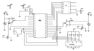
Fig. 2. Complete circuit. Description of the hardware used, showing the sensors, operational Amplifiers, electronic devices and their operating configuration, the interface between the PIC and the LCD and the input voltages required for the adequate functioning of the system.
