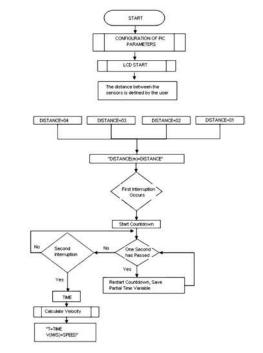
Fig. 3. Flow diagram for the microcontroller program. Indicating the sub programs [10].
