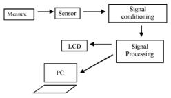
**Fig. 1.** Block diagram illustrating the basic design of the project. The sensor determines the time when the light beam is interrupted, then the elapsed time is defined to calculate the velocity by signal processing (PIC) the LCD is used to show the results.
