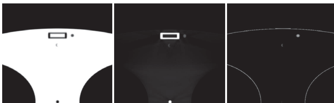
Fig.10. Fractions of water ( left), bone (center) and iodine solution 1.2% w/w (right) after the decomposition, in the noiseless case.
