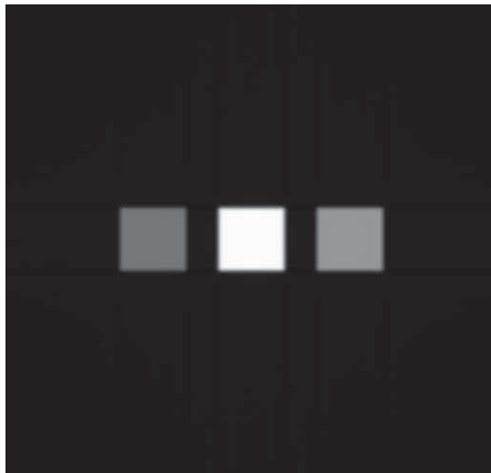
Fig.3. Calibration phantom at 120 keV. From left to right (in the boxes): water, bone and iodine solution 1.2%w/w.
