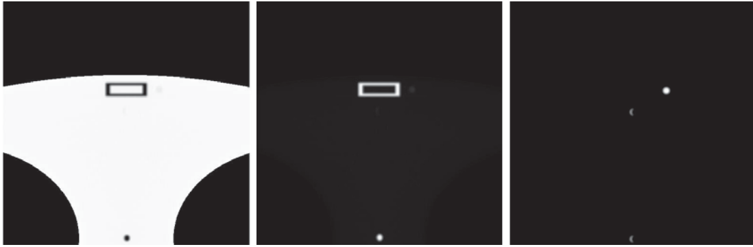
Fig.5. Fractions of water (left), bone (center) and 1.2% w/w iodine solution (right) after the decomposition, in the noiseless case.
