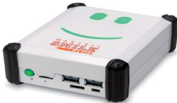
Figure 5. Adhoc local area mobile learning network – content & application server+router+wifi+storage One button and runs on a battery. Source: Author.
