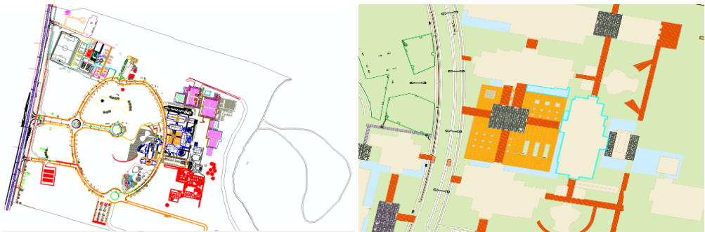
Figure 4. Left: Extraction of functional CAD layers. Right: SIG functional layers
